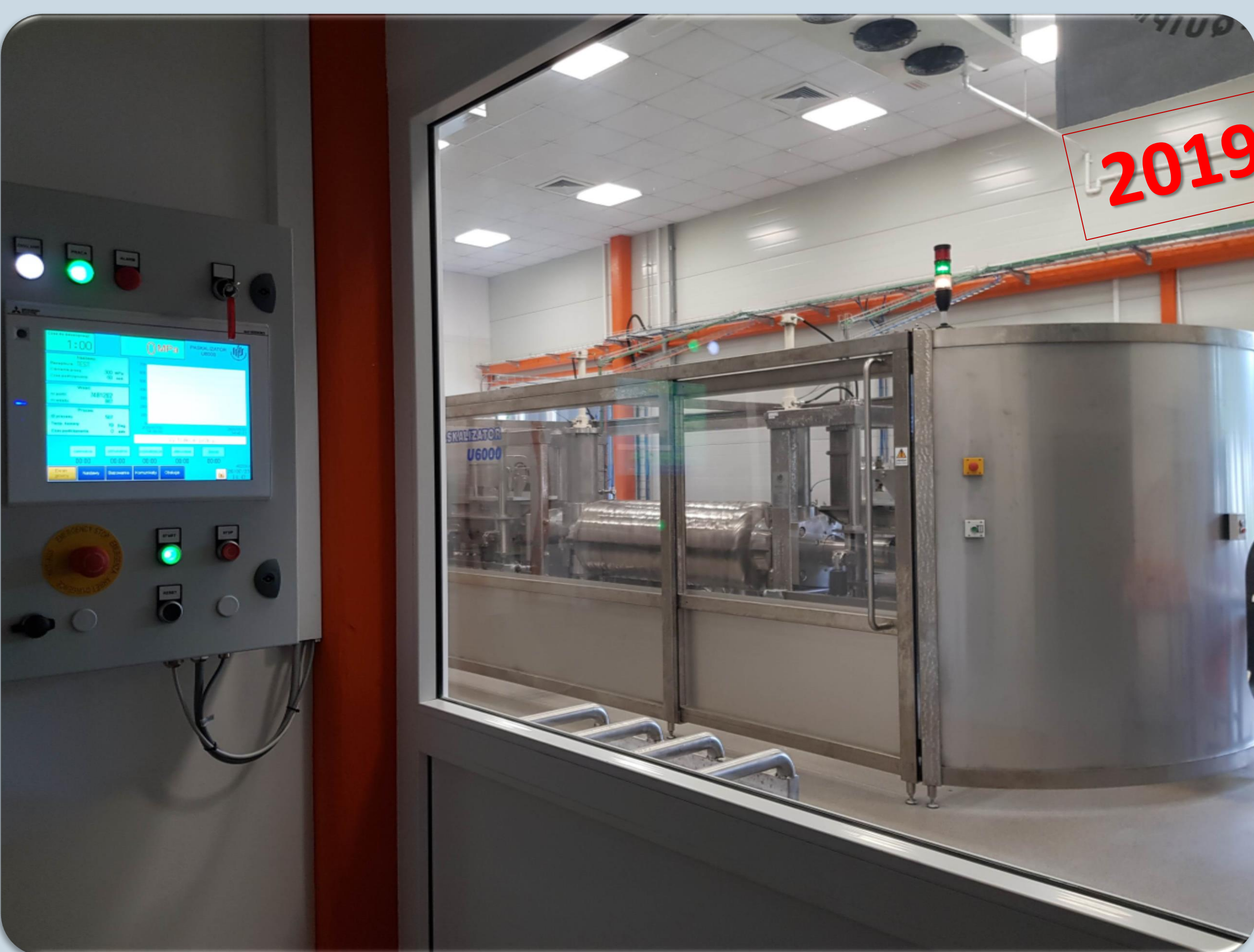
The first HPP pilot plant for food, U6000
